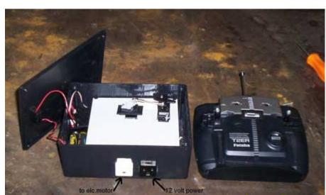
After trying and making all kinds of different ways to keep from ripping out the control cable, I made this remote control out of a RC controller and a bunch of parts. It's crude but it dose work. This one only controls the nozzle, but could be made to control the throttle also.
